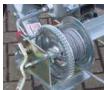
Manual winch with cable & shackle
