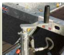
HD Jockey upgrade with locking pin
