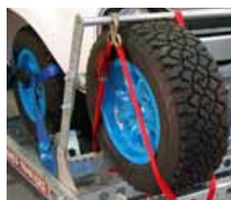
Low level tyre rack and straps
