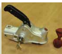
High security head with integral lock
